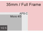
Okay, you can see that 35mm (full frame) is about twice the size of most D-SIr APS-C sensors. Micro 4/3 is slightly smaller. What is that little one doing in the lower corner? It is tiny. Why is that a popular size? That is the sensor in your bridge camera, phone, or compact point n shoot. Yes, that is why your pics from your phone are so noisy. In order to produce a viewable image from that sensor, it must be magnified many many times and with magnification comes more noticeable noise.
